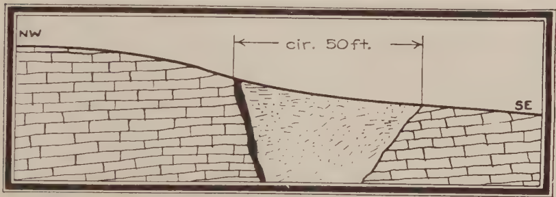
2. Illustrative of main fault and a subsidiary fissure at one point on the Larue system.
